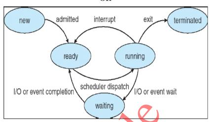
During the lifespan of a process, its execution status may be in one of four states: (associated with each state is usually a queue on which the process resides)
